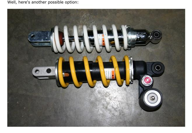
On the top is the stock '06 SV650 shock, on the bottom is the stock '06 GSXR600 shock.
