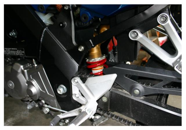
2006 SV650s - D&D, Corbin Saddle, Fender Eliminated, Flush LED Turn Signals, Progressive fork springs, 14:44 final, Speedo-Healer, GSXR600 rear shock, Scott damper.
