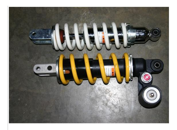
On the top is the stock '06 SV650 shock, on the bottom is the stock '06 GSXR600 s
