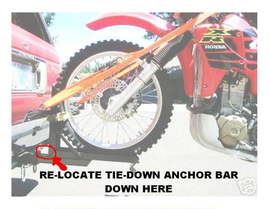
re-locate tie-down crossbar down to bottom of vertical/horizontal.
