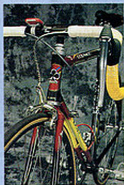
Straight-blade fork and double down tubes make Carbitubo unique on the pro circuit.
