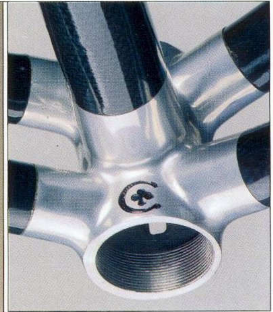
In the insert we can see not only the central gearbox, but also the frame, without fork, in which the accuracy of the details and the oblique section obtained with two twinned tubes should be noted. On the opposite page, the perfect geometry of the complete structure with the special aluminium alloy fork.
