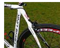
A cleanly executed wishbone-style seat stay assembly
