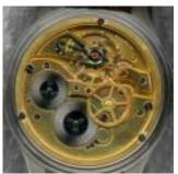
A total of 1200 cal. 5 SC (offically "52T-19" H6 S.C.") movement were made, and around 1000 went in the B-Uhr made by IWC. The cal. 52 SC was 43.15 mm (19 lignes) x 6.0 mm, 16 jewels, and 18,000 bph. The movement bore a swan-neck regulator and were adjusted in 6 position and tested at the Gesundbrunnen observatory in Glashütte. The 55 x 16.5 mm cases were numbered 1033201 1034200 and had ar additional anti-magnetic inner case.
