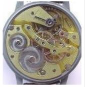
Durowe (Deutsche Uhren-Rohwerk) was part of Laco. The 22-ligne, 22-jewel movement has a ve large (22 mm) balance and a simp regulator.
