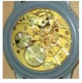
The movement has a snail-cam fine regulator.
