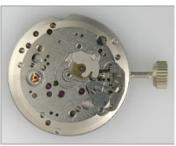
The movements are 40+ years old and were manufactured with the best possible precision at that time. We carefully disassembled, cleaned and regulated them to achieve best possible accuracy for these historical movements.
