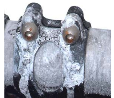
Thick salt crust after 400h hot and wet tests inside the Syntace SSM chamber.
