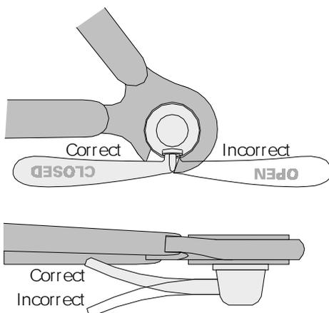
**18.35** The solid images are quick-release mechanisms as they appear when they have been closed properly by utilizing the cam (flipping the lever). The outlined levers are quick-release mechanisms as they appear when they have been secured incorrectly (as though the lever was a wing-nut).
