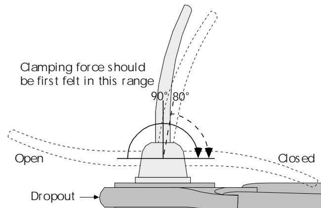
**18.36** When properly set, as the lever swings from the open to closed position, clamping force should first be felt when the base of the lever is 80-90° from the closed position (the base of the lever parallel to the dropout face).
