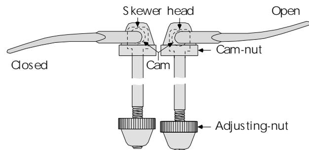
**18.1** As the lever swings from the open to closed position, it rotates the cam, which moves the skewer-head further into the cam-nut, effectively moving the cam-nut and adjusting-nut closer together (which creates the clamping force).
