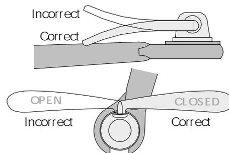
**18.24** The solid images are quick-release mechanisms as they appear when they have been closed properly by utilizing the cam (flipping the lever). The outlined levers are quick-release mechanisms as they appear when they have been secured incorrectly (as though the lever was a wing-nut).
