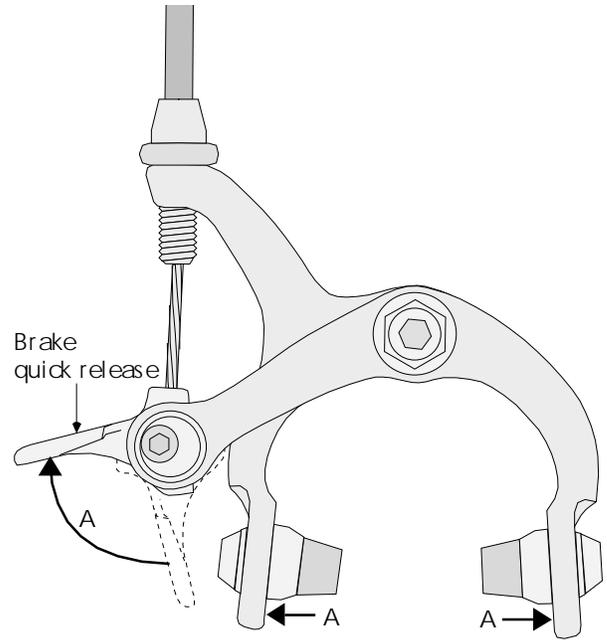
18.28 A sidepull brake should be released before installing the wheel.
