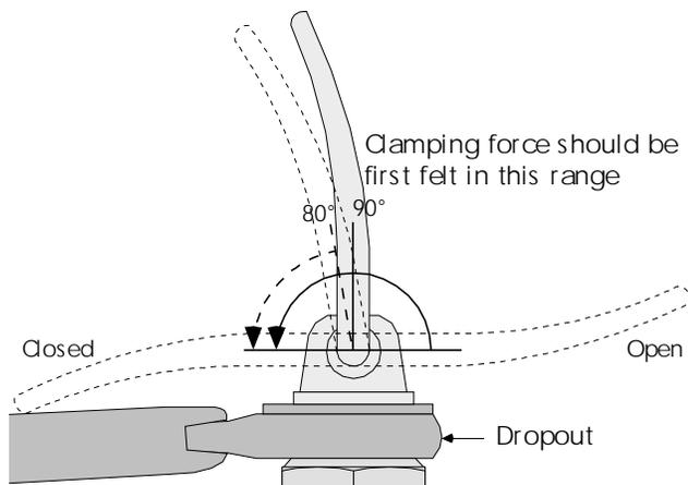
**18.2** When properly set, as the lever swings from the open to closed position, clamping force should first be felt when the base of the lever is 80-90° from the closed position (the base of the lever parallel to the dropout face).
