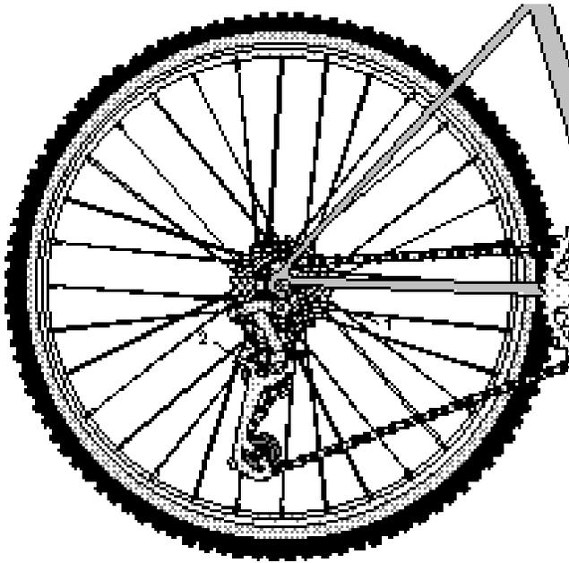
*18.34 Pull wheel back and up so that axle seats in axle slots, then allow derailleur to swing forward.*
