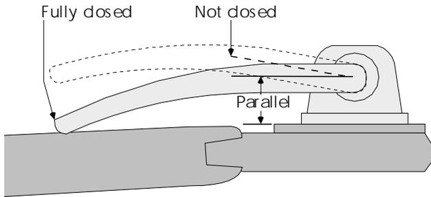
18.26 When closed, the base of the lever **must** be parallel to the dropout.
