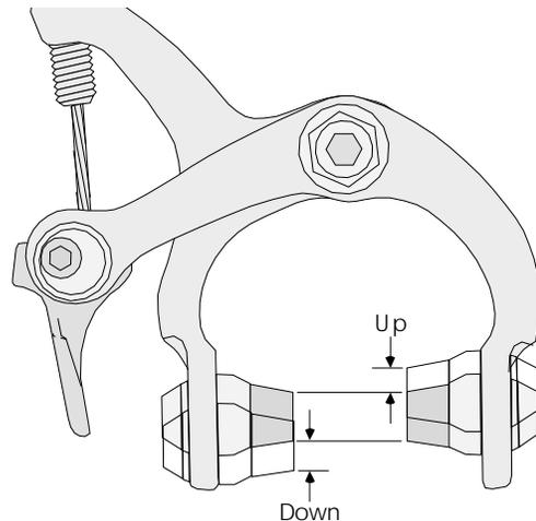
18.17 Vertical pad adjustment of a sidepull brake.
