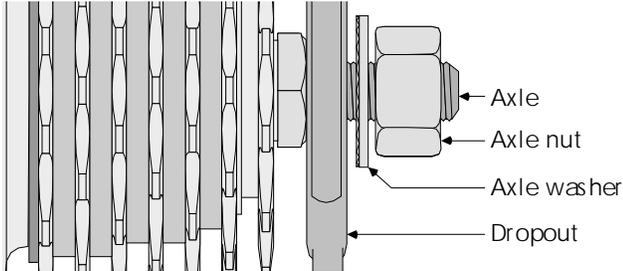
18.30 Orientation of axle nut, washer, and dropout.
