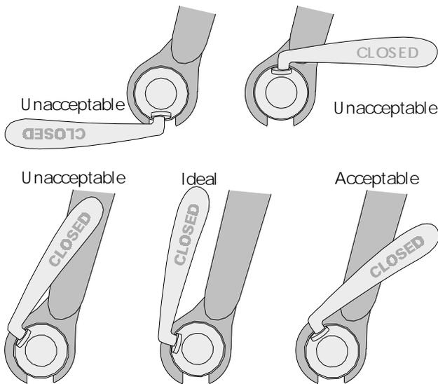
18.27 When closed, the lever should be adjacent to, but not overlapping, the fork blade.
