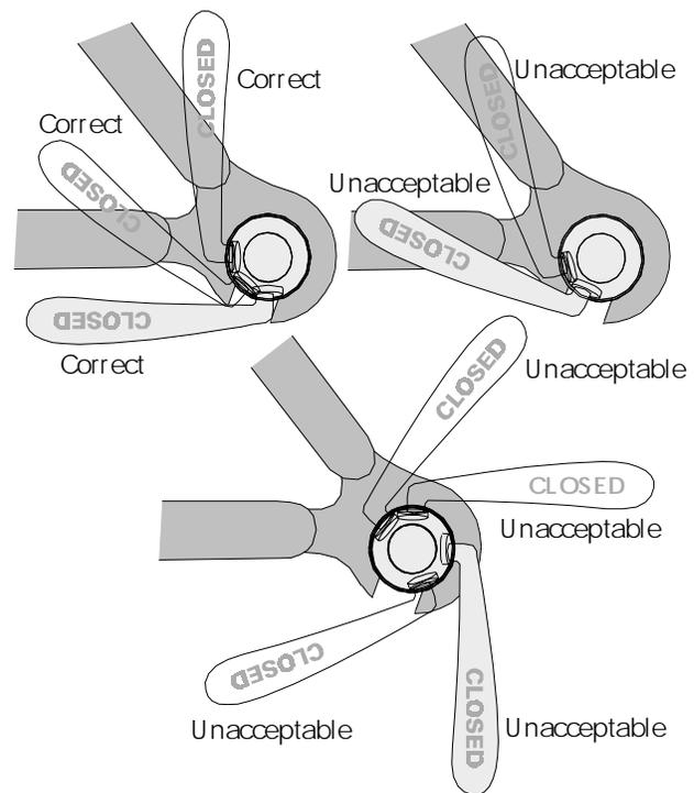
**18.38** When closed, the lever should be adjacent to, but not overlapping, the chain stay or seat stay.
