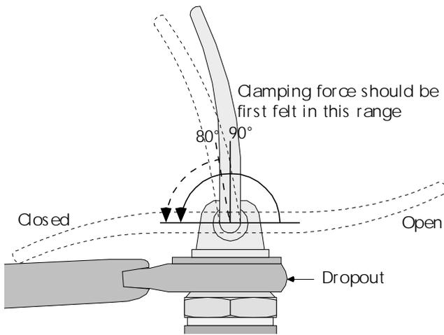
18.25 When properly set, as the lever swings from the open to closed position, clamping force should first be felt when the base of the lever is 80-90° from the closed position (with the base of the lever parallel to the dropout face).
