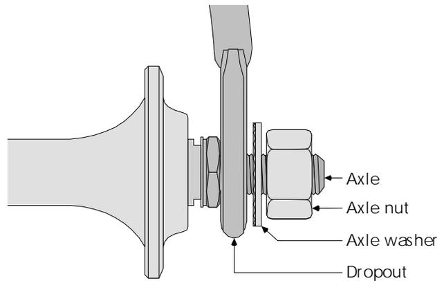
**18.22** Orientation of axle nut, washer, and dropout.
