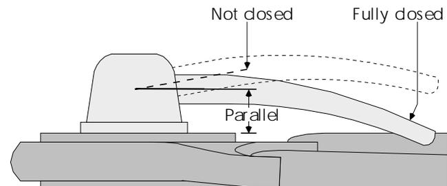
**18.37** When closed, the base of the lever **must** be parallel to the dropout.
