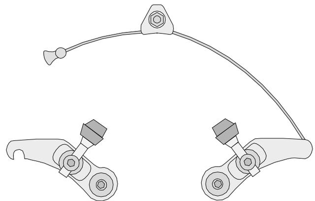
18.29 A cantilever brake should be released before installing the wheel.
