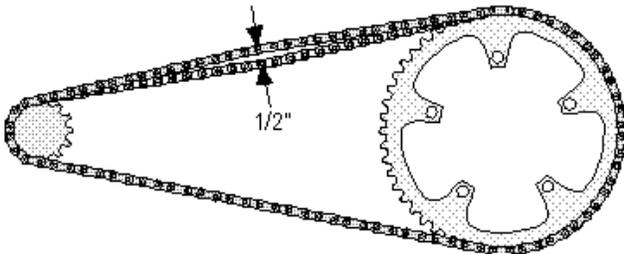
**18.39** The chain should have 1/2" of free play when the crank has been rotated to the point that puts the chain under the most tension.
