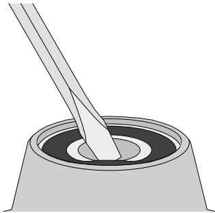
13.13 Removing the seal from the bearing.
